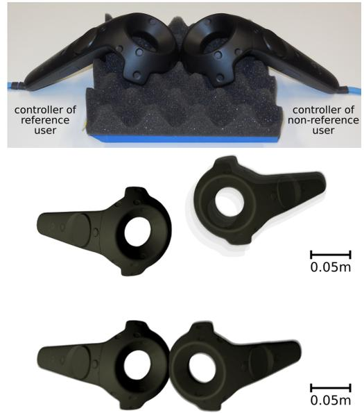
Figure 2: Hardware setup of our experiment (top) and overlaid top views of the 15 controller visualizations in the virtual environment without (middle) and with (bottom) our correction computations activated.
